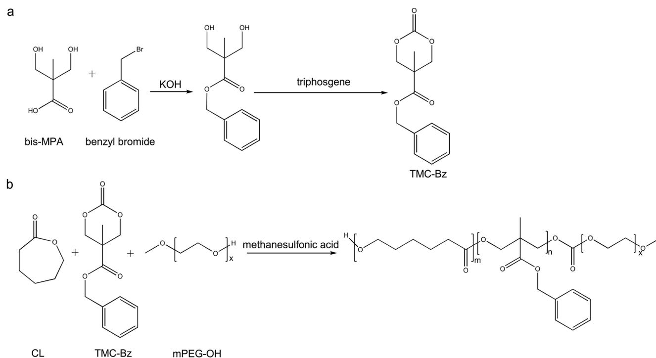
**Fig. 1. Synthesis of the TMC-Bz monomer (a) and P(CL-co-TMC-Bz)-PEG copolymer (b).** TMC-Bz, benzyl 5-methyl-2-oxo-1,3-dioxane-5-carboxylate; P(CL-co-TMC-Bz)-PEG, poly( $\epsilon$ -caprolactone)-co-poly (benzyl 5-methyl-2-oxo-1,3-dioxane-5-carboxylate).
