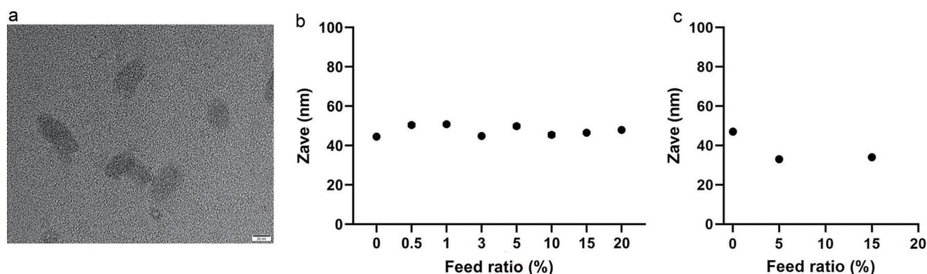
**Fig. 2. (a)** TEM image of P(CL<sub>11</sub>-co-TMC-Bz<sub>5</sub>)-PEG micelles prepared using thin-film hydration (scale bar = 20 nm), and **(b and c)** the Zave of olaparib-loaded micelles with various wt% loadings prepared using the thin-film hydration and nanoprecipitation methods, respectively. TEM, transmission electron microscopy; Zave, Z-average hydrodynamic diameter.
