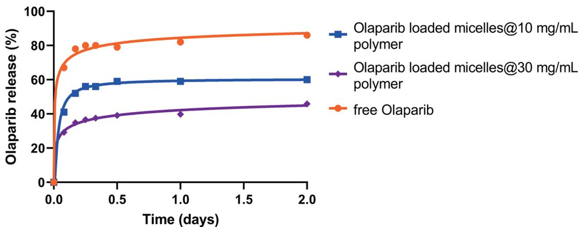
**Fig. 4.** Release profiles of olaparib-loaded polymer micelles and free olaparib obtained in PBS (pH 7.4) supplied with 0.5% Tween-80 at 37°C.
